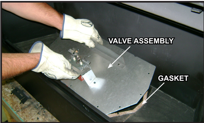
Figure 16.6 Remove Valve Plate
